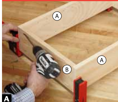
A Position the ends of the sides (A) flush with the faces of the top and bottom (B). Drive coarse-thread pocket-hole screws.
